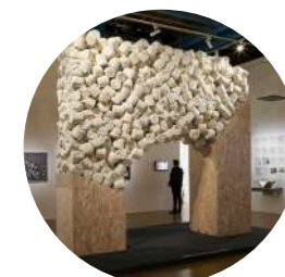
Living Bricks, The Living, 2019 In-situ growth of the material to bond individual units
