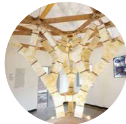
Mycotree, 2017 Moulded spatial branching structure with load-bearing mycelium components working in compression
