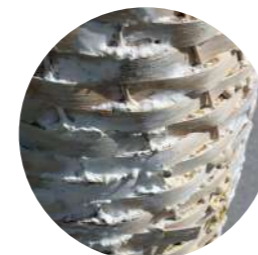
House Parts, MycoMatters Lab, 2021 Mycelium panels grown in wooden frames
