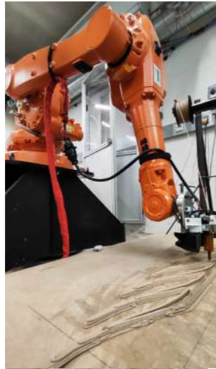
Robotically 3D printing referencing semi-support structure
