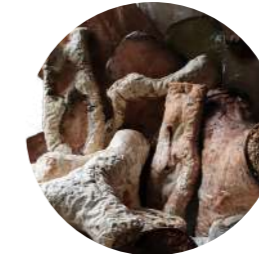
MYCOLlulose, Piórecka, Bio-ID 2022 Cotton fabric and Bacteria cellulose as sacrificial mold for mycelium
