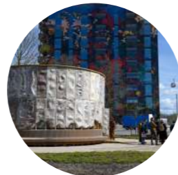
The Growing Pavilion, Krown Design, 2019 Structure combining light, well insulative (temperature and sound) mycelium panels with a variety of organic materials
