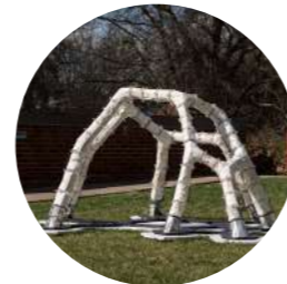
MycoCreate 2.0, Gürsoy, 2022 Spider-like legs, made using moulded blocks of mycelium for branching structure that supports fungi.
