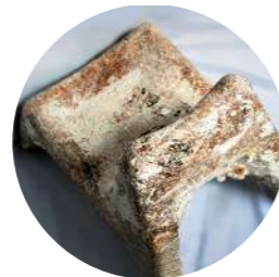
MYCOsella, Piórecka 2017 Exploration of structural capacity of mycelium as a chair topology, using reusable moulding fabrication
