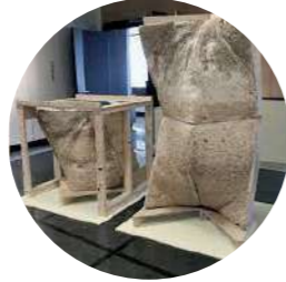
L'Orso Fungino, MycoMatters Lab, 2021 Upholstered formwork with synthetic geotextile fabric
