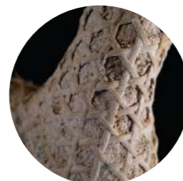
Generated Kagome Morphologies, CITA, 2021 The weave acts as a combined stay-in-place formwork and reinforcement.
