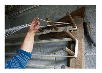
To warp is to dispose the threads of the web in an organized way, according to its length and to be later mounted on the loom.
