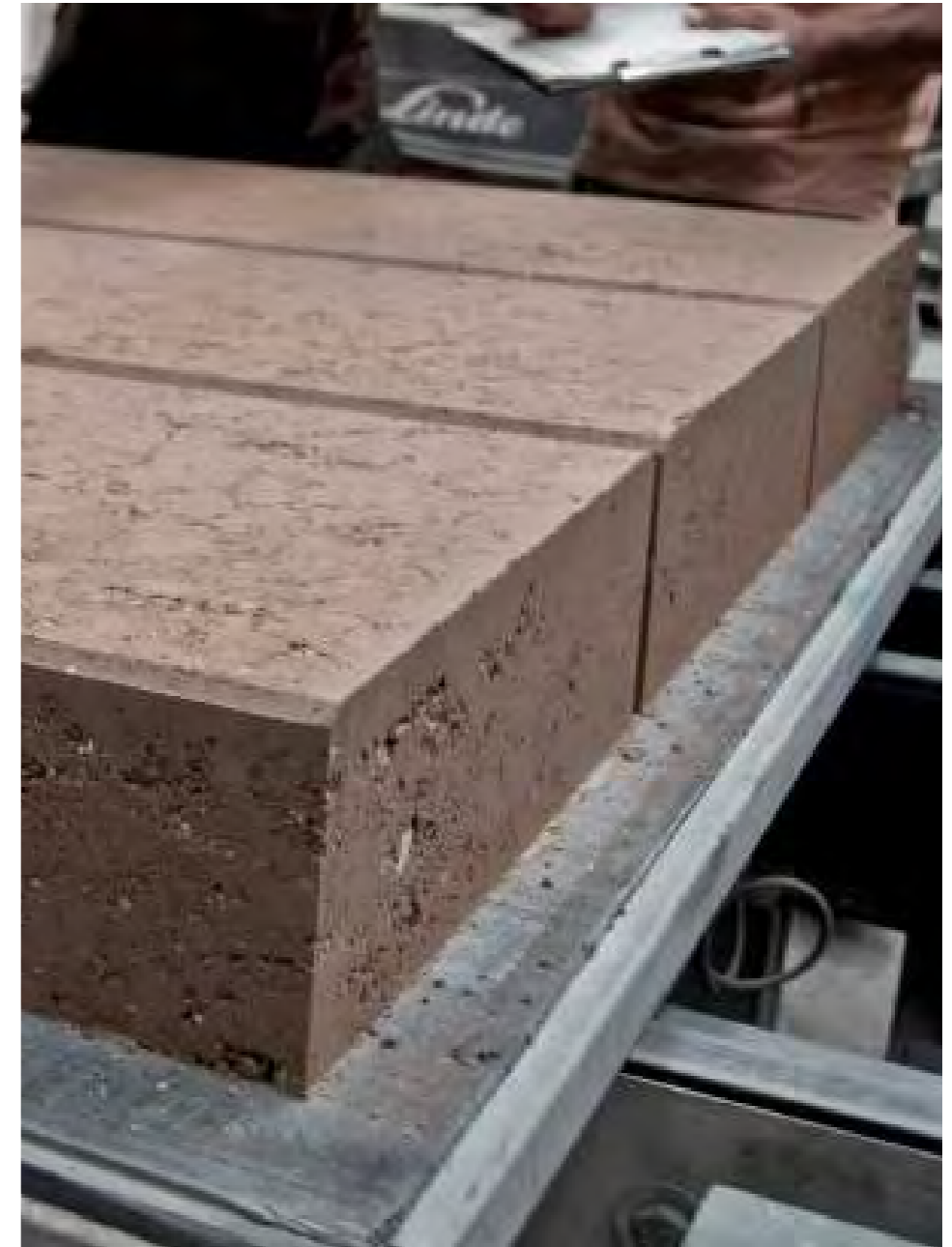
PREFABRICATED COMPRESSED RAMMED EARTH
