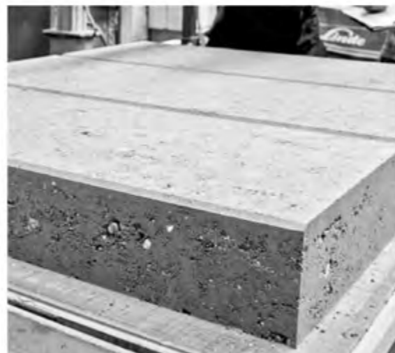
COMPRESSED RAMMED EARTH (PREFABRICATED UNITS)
